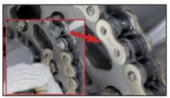
9a. With the inside of the connecting link pushed into place holding the chain together with the pins sticking out the outside of the chain, slide the O-Rings/X-Rings® into place and temporarily press the other side plate on the pins by hand. Set the Cutting pin location on your chain tool's U-shaped holder to the point A position.
