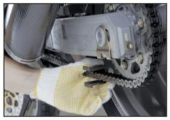
Ia. Before cutting your chain, loosen it using your motorcycle's rear wheel adjusters. Position your KM500R or KM501E over your chain on the bottom side of your swingarm; cut the pin on the right side of the link you choose first. If your chain has a master link, it is easier to cut the chain at the master link.
