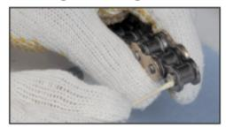
8a. Before installing the connecting link, be sure to put a heavy coat of the supplied grease into the holes of the bushings of the new chains' links, and on the surface of the connecting link's pins. If you are installing an O-Ring or X-Ring® chain, don't forget to put heavily greased O-Rings or X-Rings on the pins between the side-plates on both sides of the chain.
