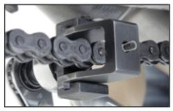
5a.Turn 19mm wrench clockwise on the tool's Hexagon bolt head to push the pin completely out.
