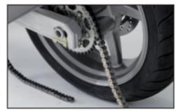
6a. After pushing the pin out, disassemble the chain tool from the chain.
